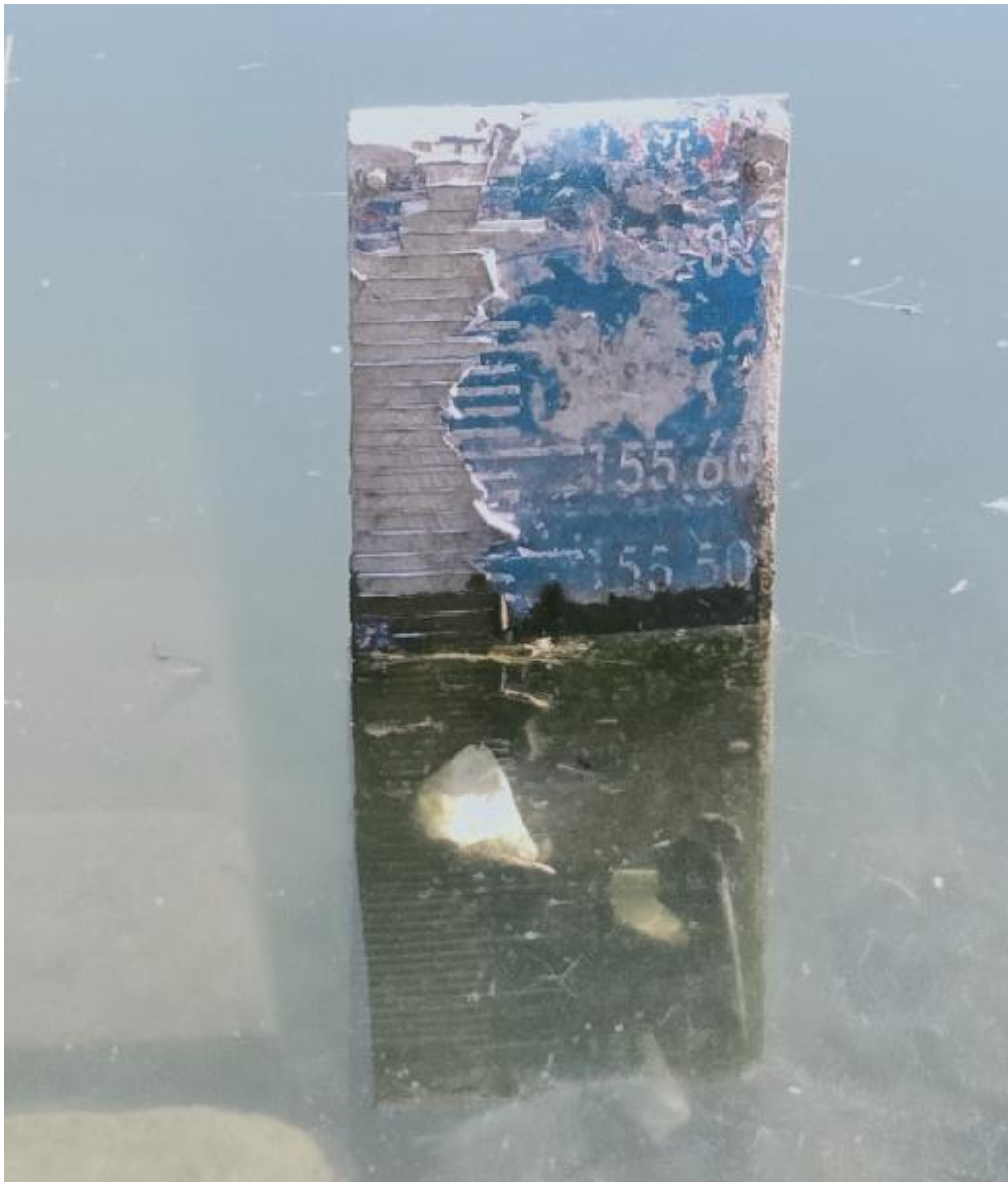
WATER LEVEL GAUGE
